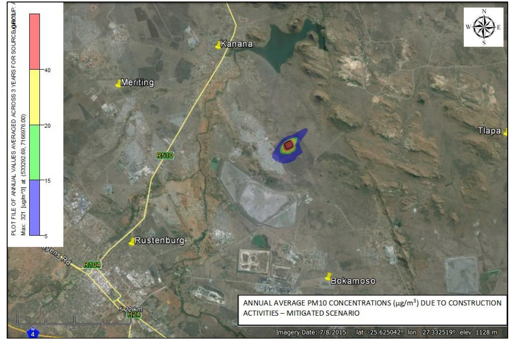
FIGURE 5-23: ANNUAL AVERAGE PM10 CONCENTRATIONS ( \mu\text{G}/\text{M}^3 ) DUE TO CONSTRUCTION ACTIVITIES AT THE EXTENSION SITE (MITIGATED).
