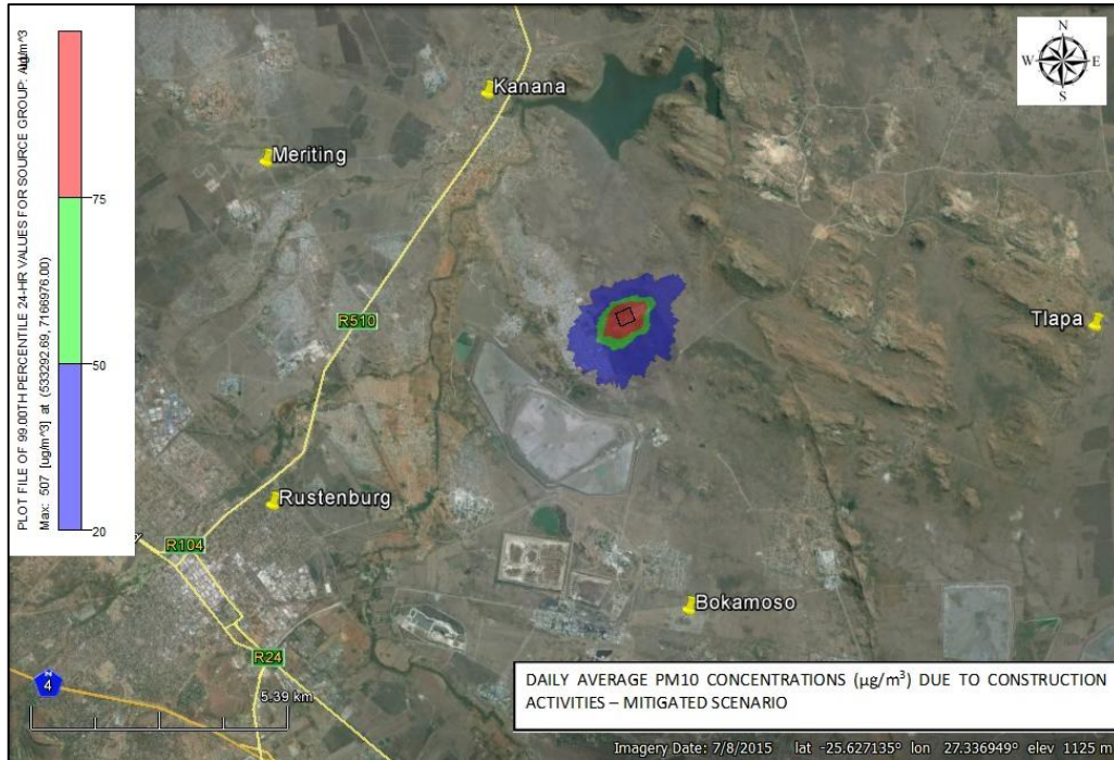
FIGURE 5-22: DAILY AVERAGE PM10 CONCENTRATIONS ( \mu\text{G}/\text{M}^3 ) DUE TO CONSTRUCTION ACTIVITIES AT THE EXTENSION SITE (MITIGATED).
